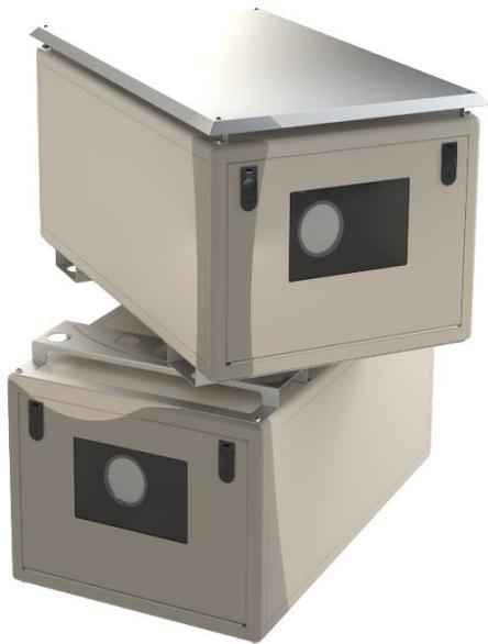
Tempest has developed a sun shade accessory for G4 enclosures, and tests are ongoing. The purpose of the sun shade is to reflect sunlight from the top of the enclosure and introduce an air gap, with convected air movement, to mitigate enclosure heating when exposed to strong sunlight.
